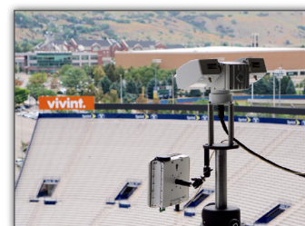
Figure 12-13 - UAVX mounted on tripod at skybox-level with thermal camera system and radar
