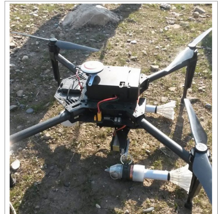
This drone was used by Iraqi government forces against ISIS in Mosul. It shows the the weapon carriage and arming method, using two attachments. The weapons are maintained safe and could be armed just before takeoff.
