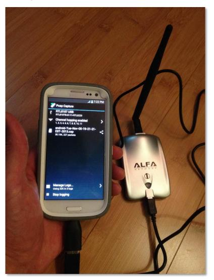
Model Number AWUS036H. This uses the RTL8187 Wireless Chipset.
