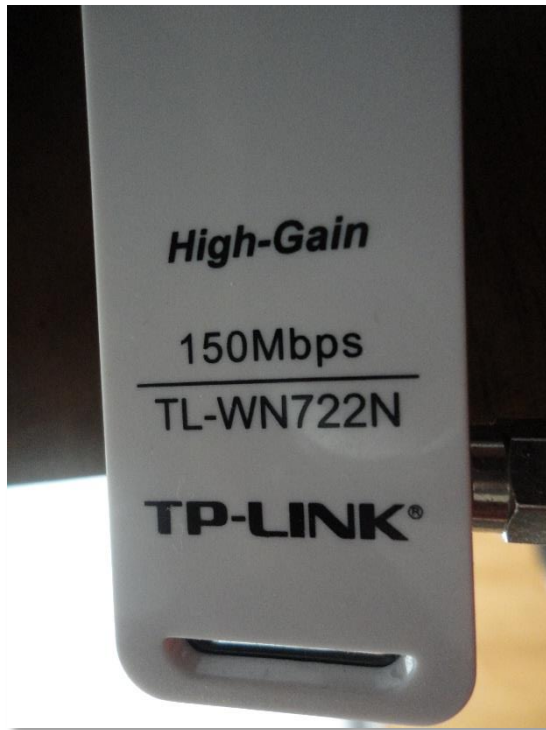
TP-Link Adapter Capable of attaching a YAGI antenna
